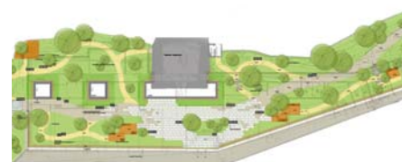
The draft plan shows how the roof garden is integrated into the surrounding landscape. A path which is accessible even with smaller maintenance vehicles crosses the entire roof.
